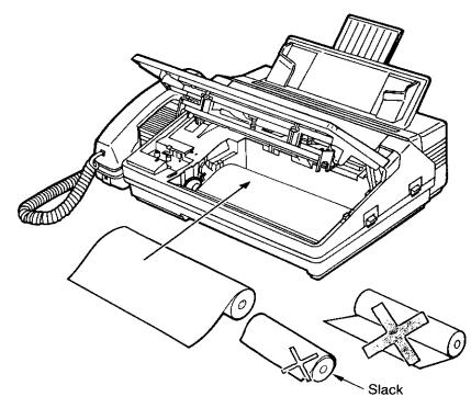
Insert the recording paper between the upper and the lower guide plates and pull the paper a few centimeters (one or two inches) out of the unit.
